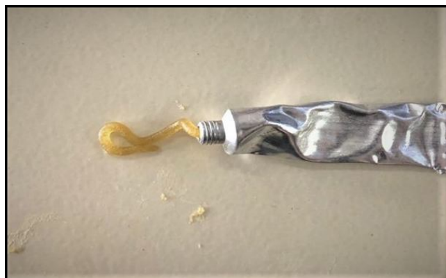
Fig. 2: Extrudability test showing best result.
